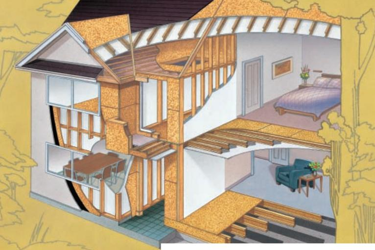
The consistent quality of *AinsworthEngineered* osb is available in different grades for wall and roof sheathing and flooring.
